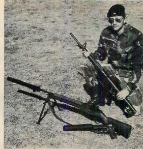
Rhodesian soldier poses with silenced Colt .45, M-14 with Sionics-type suppressor, and 7.62 caliber AR-10 assault rifle.
